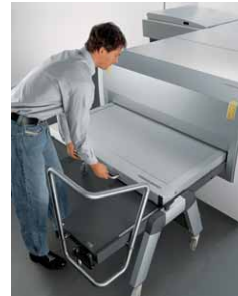
Once the cassette has been unlocked, it can be inserted easily into the loader. The plates are then fed automatically to the recorder.
